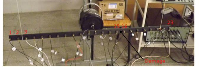
Fig. 1. Experimental setup with the identification of the accelerometers and damage location.
