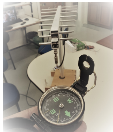
Fig. 7. Proposed antenna electronic tracking system for full channels reception in 46.8^\circ north east direction.
