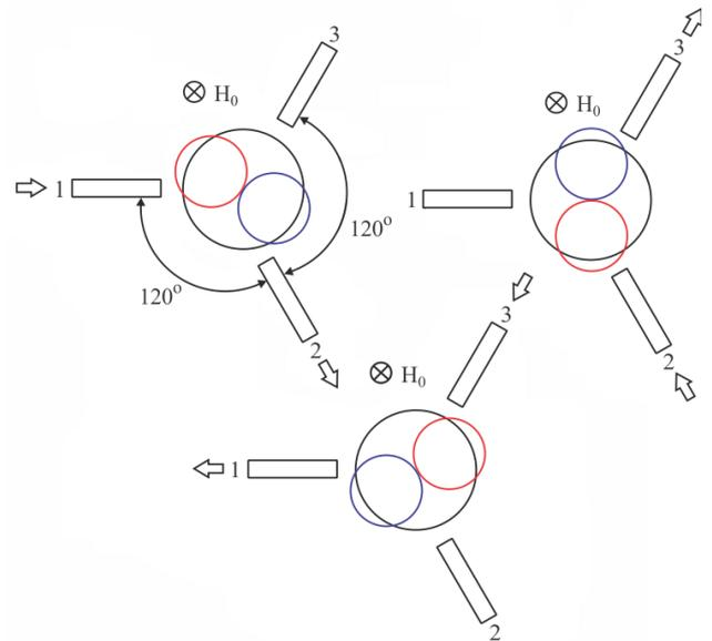
Fig. 1. Schemes of the three-port optical Y-circulator excited at each port with the dipole mode in the cavity. Direction of circulation is  $1 \rightarrow 2 \rightarrow 3 \rightarrow 1$ .
