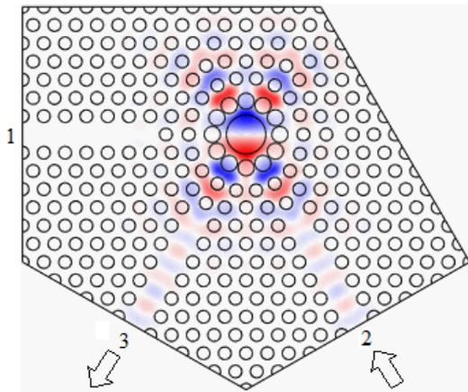
Fig. 8. Simulated  $H_z$  amplitude of the W-circulator for excitation at port 2.
