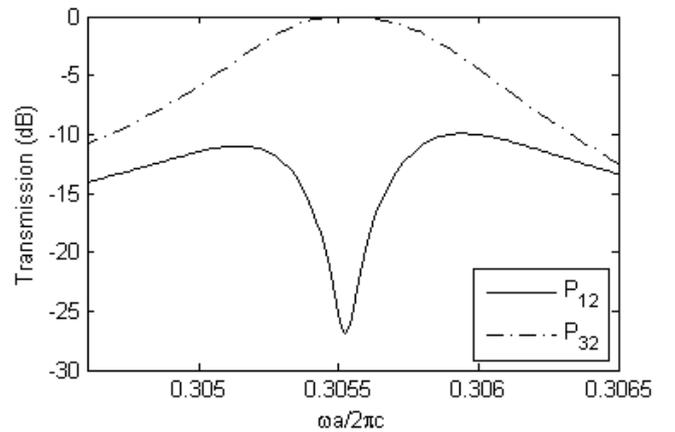
Fig. 4. Power transmission and isolation curves for excitation at port 2.
