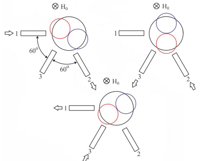
Fig. 2. Schemes of the three-port optical W-circulator excited at each port with the dipole mode in the cavity. Direction of circulation is  $1 \rightarrow 2 \rightarrow 3 \rightarrow 1$ .
