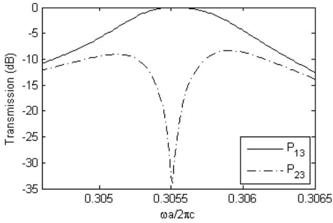
Fig. 5. Power transmission and isolation curves for excitation at port 3.
