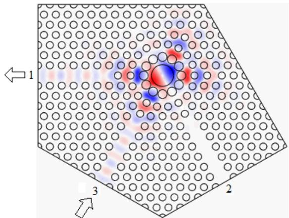
Fig. 9. Simulated  $H_z$  amplitude of the W-circulator for excitation at port 3.
