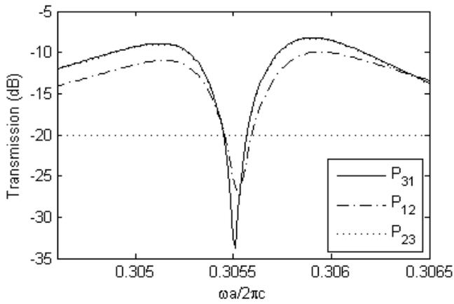
Fig. 6. Isolation curves for excitation at ports 1, 2 and 3.
