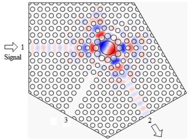
Fig. 7. Simulated  $H_z$  amplitude of the W-circulator for excitation at port 1.
