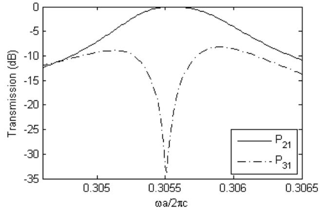
Fig. 3. Power transmission and isolation curves for excitation at port 1.
