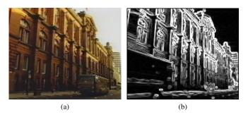
Fig. 1: Effect of the gradient vectors computed by Sobel operators
