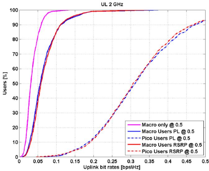
Fig. 6. Uplink bit rates for the reference case.
