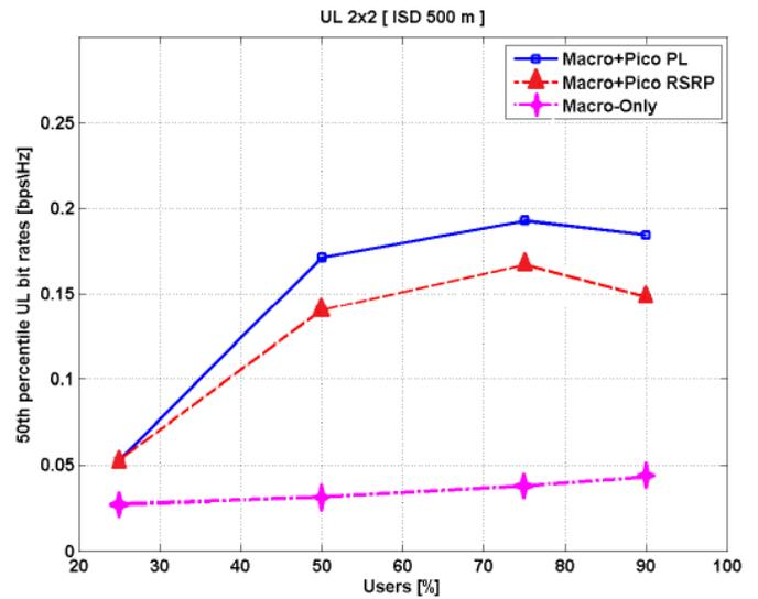
Fig. 11. 50<sup>th</sup> percentile of uplink bit rates for different systems and hotspot densities.
